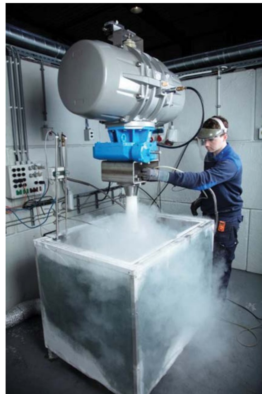
Testing the stem seal of a cryogenic valve using a helium detector with sniffer probe.
