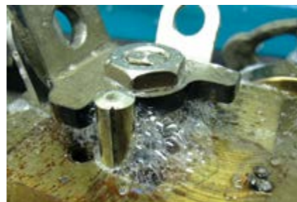
Stem seal leakage after high-temperature testing.
