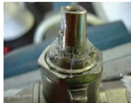
Stem seal failure after a few operational cycles at room temperature.
