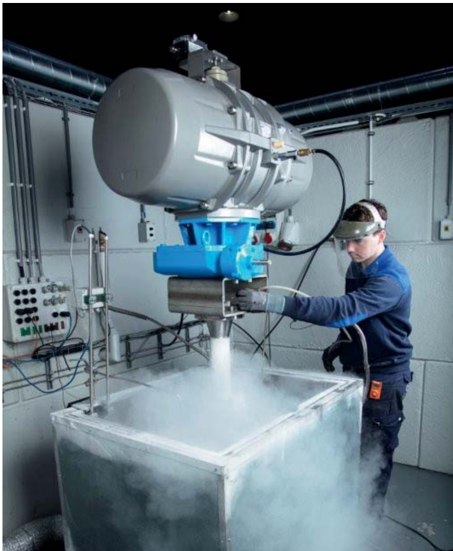
Testing the stem seal of a cryogenic valve using a helium detector with sniffer probe.
