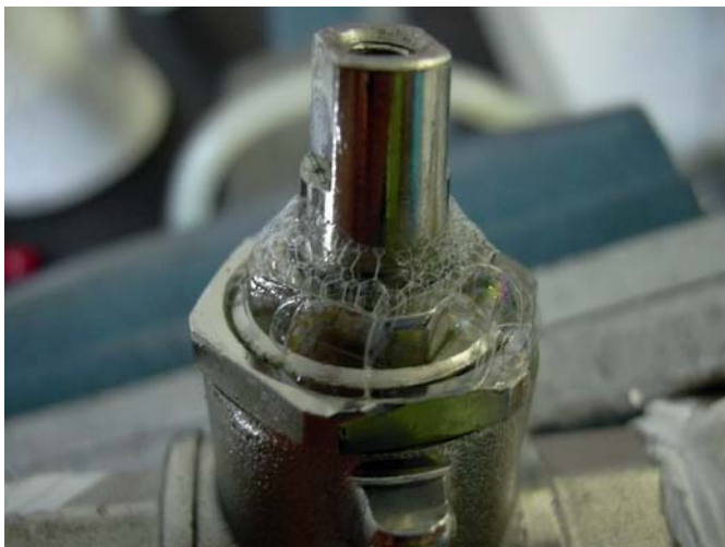
Stem seal failure after a few operational cycles at room temperature.
