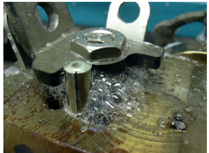
Stem seal leakage after high-temperature testing.
