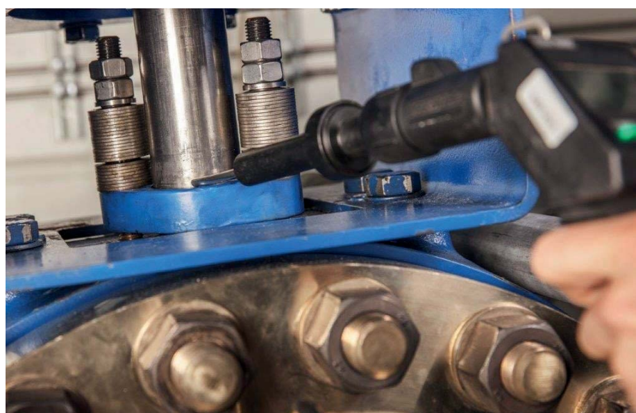
Testing a stem seal with 'live loading', using methane as the test medium and an FID leak detector.
