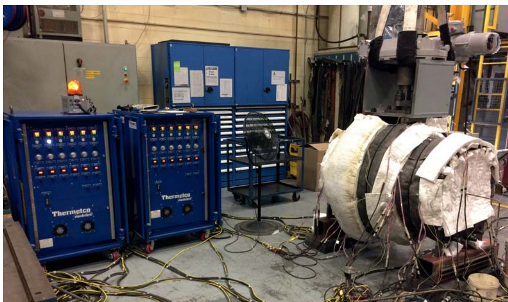
Design Validation Testing on a NPS 24 ASME Class 300 Velan metal-seated ball valve at over 400 Deg C.
