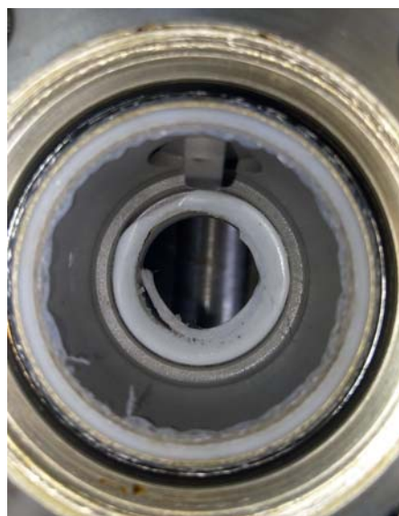
Melted PTFE seats of a ball valve after a DVT test. Tested at 200°C and 50 bar nitrogen.
