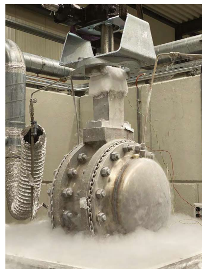
Butterfly valve after a DVT test. Tested at cryogenic conditions (-196°C).
