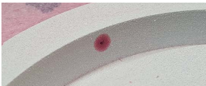
Dye penetrant testing can reveal defects, such as in this RTJ end flange on a valve body
