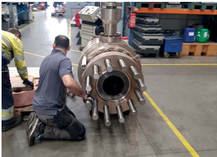
Following an overhaul, valves need to be tested. Image shows blind flanges being fitted to enable hydro testing and seat testing
