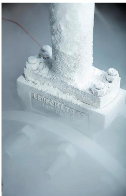
Cryogenic flange testing being carried out
