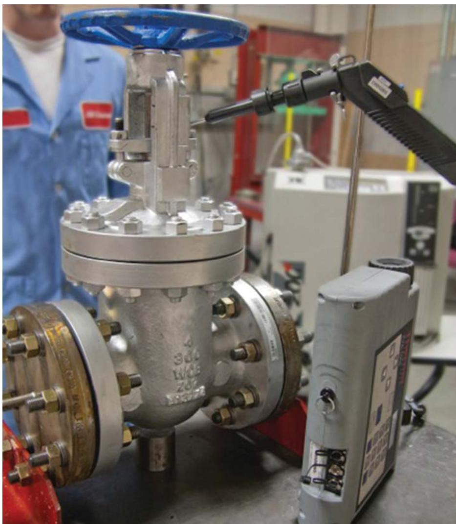
to measure and certify static and dynamic leakage values. Specific leakage rate limits for these seals are stated in VDI 2440. The values are  $10^{-4}$  mbar\*l/(s\*m) at temperatures < 250°C (482°F) and  $10^{-2}$  mbar\*l/(s\*m) at temperatures > 250°C. These leak rates must be maintained permanently.
