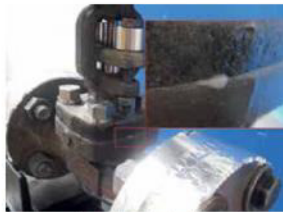
Leaking valve during hydrostatic and FE testing
