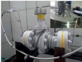
Leakage of an O-ring at low temperatures
