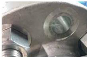
Crack in valve body casting
